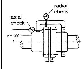
Radial: max. 0.05 mm shaft misalignment (i.e. 0.1 mm total full revolution).
